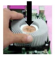
3. Mount the fan on top of the heatsink. Press down the fan until its four clips get wedged in the holes of the retention mechanism.
